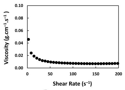
**Figure 7.** Viscosity of the  $^{152}$ Sm<sub>2</sub>(CO<sub>3</sub>)<sub>3</sub>-PMA microsphere suspension at a concentration of 2.5% (w/v). The viscosity was measured in saline solution of 37 °C at various shear rate.
