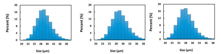
**Figure 3.** Particle size distribution of  $^{152}$ Sm<sub>2</sub>(CO<sub>3</sub>)<sub>3</sub>-PMA microspheres before (**A**) and after 6 h (**B**) and 18 h (**C**) neutron activation.
