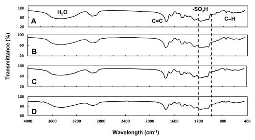
**Figure 5.** FTIR spectrum of the PMA microspheres (**A**),  $^{152}$ Sm<sub>2</sub>(CO<sub>3</sub>)<sub>3</sub>-PMA microspheres both before and after neutron activation (**B**,**C**), samarium carbonate (**D**).
