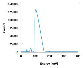
Figure 1. Gamma spectrum of <sup>153</sup>Sm<sub>2</sub>(CO<sub>3</sub>)<sub>3</sub>-PMA microspheres at 24 h after neutron activation.
