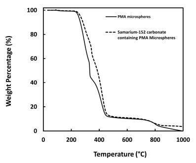
Figure 6. TGA profile of PMA microspheres (A) and <sup>152</sup>Sm<sub>2</sub>(CO<sub>3</sub>)<sub>3</sub>-PMA microspheres.
