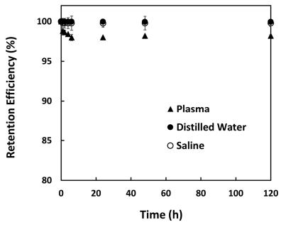
**Figure 8.** Retention (%) of  $^{153}$ Sm in  $^{152}$ Sm $_2$ (CO $_3$ ) $_3$ -PMA microspheres suspended in distilled water, saline solution and human blood plasma over 120 h.
