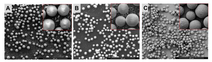
**Figure 2.** Scanning electron images of the  $^{152}\text{Sm}_2(\text{CO}_3)_3$ -PMA microspheres both before (**A**) and after 6 h (**B**) and 18 h (**C**) neutron activation.
