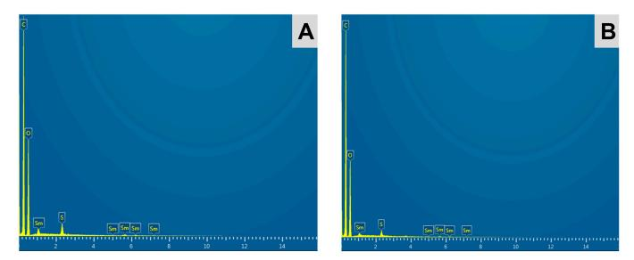
**Figure 4.** EDX spectra of the  $^{152}$ Sm<sub>2</sub>(CO<sub>3</sub>)<sub>3</sub>-PMA microspheres both before (**A**) and after neutron activation (**B**), showing the presence of carbon (C), oxygen (O), sulphur (S) and samarium (Sm) elements in the samples.
