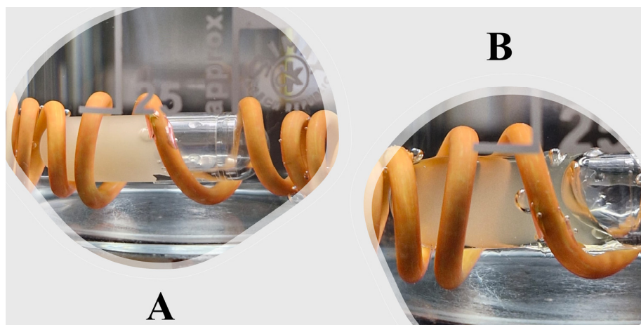
Figure 7. Surfactant-enriched cross-linked scaffold during physiological assessment that presents at (A) solid and (B) liquid state at the beginning and after incubation, respectively.
