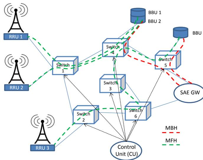
**Figure 14.** Possible architecture for converged metro-access MBH/MFH network.
