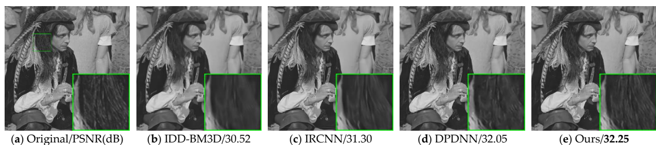
Figure 7. Image deblurring results on Man in Figure 3 with 19 \times 19 motion blur kernel and \sigma_n = 2.55 . (a) The original image. (b) The result of IDD-BM3D. (c) The result of IRCNN. (d) The result of DPDNN. (e) Our result.
