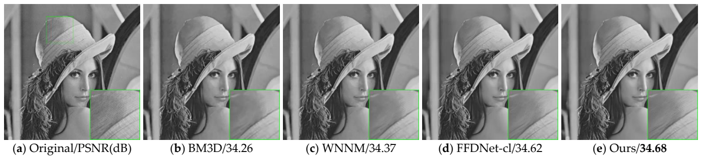
Figure 4. Image denoising results on Lena with noise level \sigma_n = 15 . (a) The original image. (b) The result of BM3D. (c) The result of WNNM. (d) The result of FFDNet-cl. (e) Our result.
