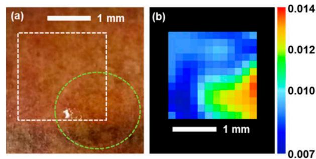
**Figure 5.** (a) Photograph of the apple peel with methomyl stain (green dashed circle). The white dashed line is the positioned nano-slot-antenna region. (b) Normalized THz reflection image taken through the nano-slot-antenna attached to the apple peel sample with a residual methomyl stain. (Reprinted/Adapted) with permission from [84] © 2016, IEEE.
