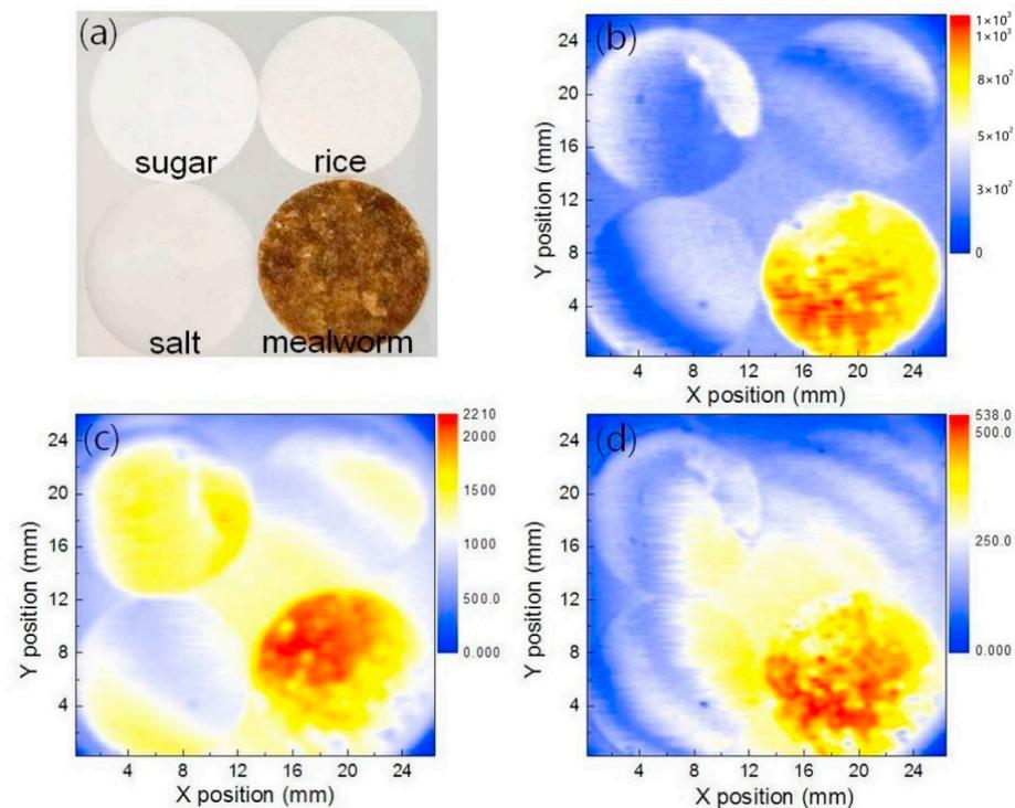
**Figure 6.** (a) The optical image of rice, sugar, salt, and mealworm pellet samples and their reflective THz images at THz frequency of (b) 1 THz, (c) 0.5 THz, and (d) 1.2 THz. (Reprinted/Adapted) with permission from [93] © 2017, Elsevier Ltd.
