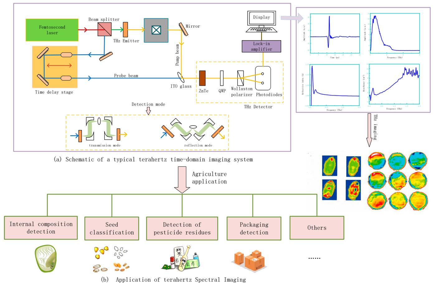
Figure 1. THz spectral imaging system and applications.
