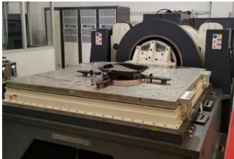
Figure 17. Vibration test of the secondary mirror assembly in the Y direction (lateral). The mirror surface is covered by a protective layer. The accelerometer was attached on the back surface of the mirror.
