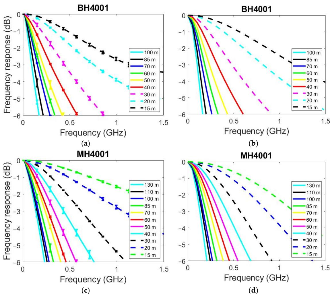
**Figure 4.** Normalized frequency response at selected fiber lengths. (a,c) Normalized frequency response measurements for BH4001 and MH4001 fibers respectively, (b,d) Normalized frequency response modeled results for BH4001 and MH4001 fibers respectively.
