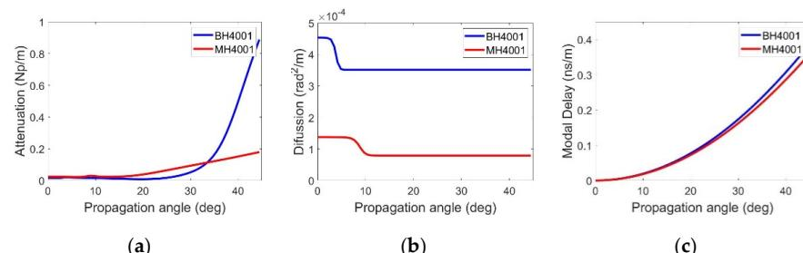
**Figure 3.** Plastic optical fiber characteristic functions as a function of the propagation angle. (a) Attenuation, (b) diffusion, and (c) group delay.
