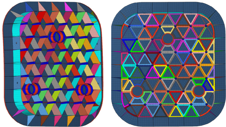
Figure 6. Lightweight ribs grouped according to their geometric position characteristics and marked with the same color.
