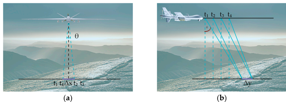
Figure 3. Diagram of micro-displacement and angle. (a) The change in the boresight in the cross-sectional view of flight direction; (b) the change in the boresight in the side view of flight direction.
