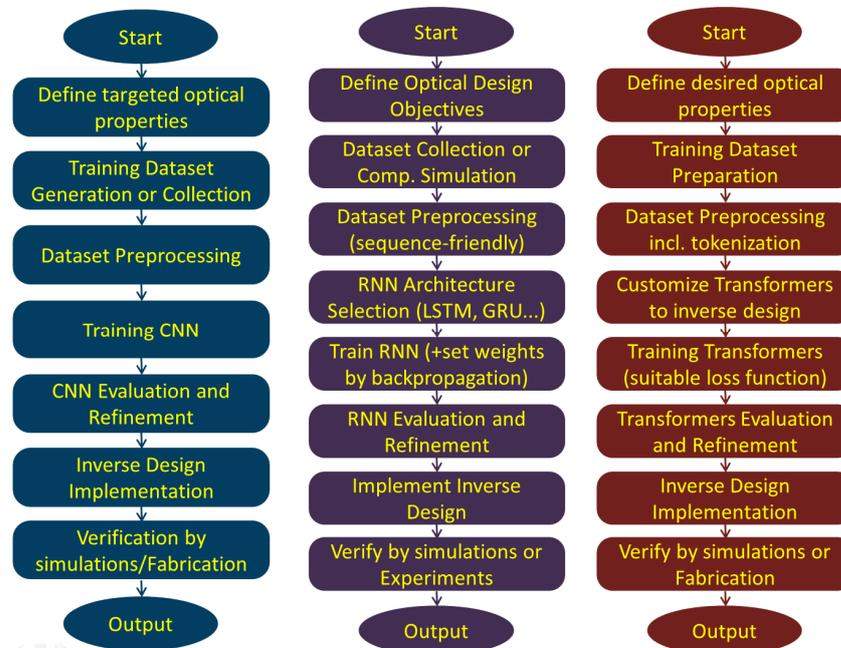
**Figure 20.** Flowcharts of inverse design of metasurfaces using three types of DNNs. **(Left):** Generic flowchart of CNN-based inverse design. **(Middle):** RNN-based inverse design flowchart. **(Right):** Transformer Neural Network-based inverse design flowchart.
