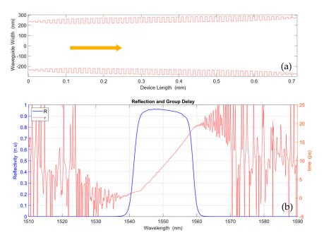
**Figure 6.** (a) Conceptual diagram of the apodized chirped IBG designed via waveguide width variation; initial width  $W_{0i} = 435$  nm and final  $W_{0f} = 546$  nm,  $L = 2258\Lambda_B$ ,  $\Delta W = 10$  nm, constant  $\Lambda_B = 316$  nm and tanh as apodization function (grating period and corrugation width sizes have been enlarged for the sake of illustration). (b) Simulated spectrum of reflectivity and group delay (GD).
