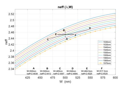
**Figure 3.** Effective refractive index obtained with numerical simulations as a function of waveguide width for different wavelengths from 1530 nm to 1570 nm (the discrete step width is 10 nm; for convenience, the sampling is marked only on the 1570 nm curve).
