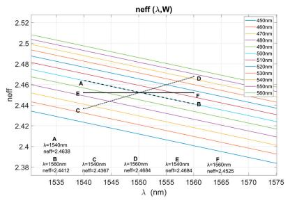
**Figure 2.** Effective refractive index obtained with numerical simulation as a function of wavelength (the discrete step wavelength is 2 nm) for different waveguide widths from 450 nm to 560 nm.
