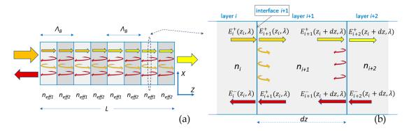
**Figure 4.** (a) Illustrative diagram of an IBG, showing incoming (orange), transmitted (yellow), and reflected (red) fields. (b) Schematic representation of the IBG sampling, and distribution of transmitted and reflected fields in a layer of size dz limited by two interfaces.  $L = dz \times n$  (n, number of layers).
