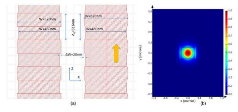
**Figure 1.** (a) Diagram of two Integrated Bragg Gratings (IBGs) with rectangular and sinusoidal corrugations and  $\Delta W = 20$  nm. The yellow arrow indicates the direction of propagation of the electromagnetic field. (b) Energy density distribution (normalized) of the quasi-transverse electric (TE) mode inside the strip waveguide (linear scale).
