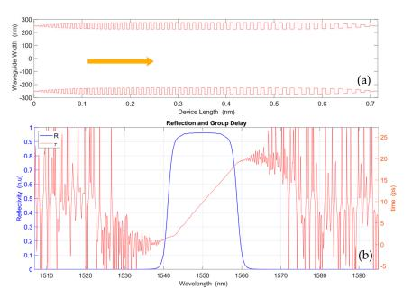
**Figure 5.** (a) Conceptual diagram of the apodized chirped IBG designed via Bragg grating period variation: initial Bragg period  $\Lambda_{Bi} = 312.5$  nm and final  $\Lambda_{Bf} = 319.5$  nm,  $L = 2258\Lambda_B$ ,  $\Delta W = 10$  nm,  $W_0 = 500$  nm, with *tanh* as the apodization function (grating period and corrugation width sizes have been enlarged for the sake of illustration). (b) Simulated spectrum of reflectivity and GD.
