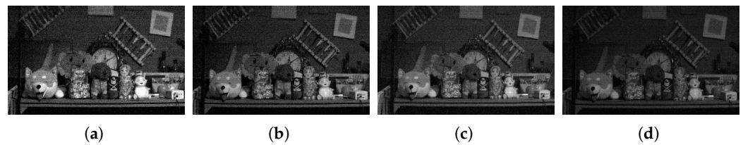
Figure 16. Comparison of different frequencies in the gating mode in an indoor environment. Exposure time T = 10 ms. (a) Picture of frequency 40 MHz. (b) Picture of frequency 20 MHz. (c) Picture of frequency 10 MHz. (d) Picture of frequency 4 MHz.
