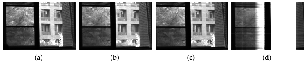
Figure 14. Comparison of different frequencies in the gating mode with an exposure time of T = 10 ms in an outdoor environment. (a) Picture of frequency 40 MHz. (b) Picture of frequency 20 MHz. (c) Picture of frequency 10 MHz. (d) Picture of frequency 4 MHz.
