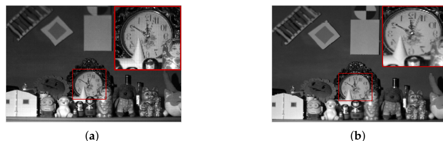
Figure 15. Pictures captured in high-brightness scenes by the free-running and gating chips with an exposure time of 10 ms. The red box highlights the region where the two pictures differ in SNR, showing the impact of the imaging mode. (a) Photo captured by the free-running chip (b) Photo captured by the gating chip.
