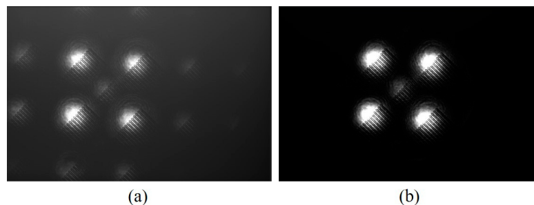
Figure 5. Experimental results of coaxial holographic two-dimensional imaging. (a) Imaging results without an aperture. (b) Imaging results with an aperture.
