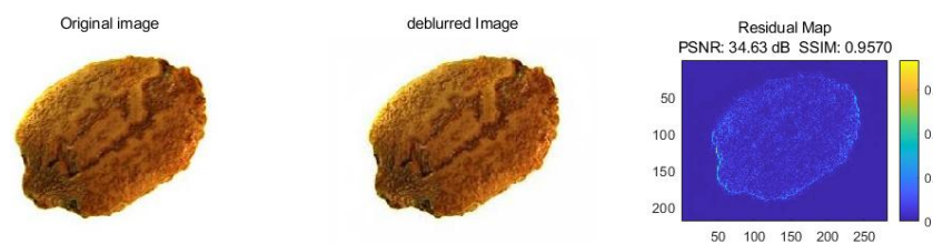
Figure 15. Original bitter melon seed image and deblurred result and residual map of the conditional generative adversarial network.
