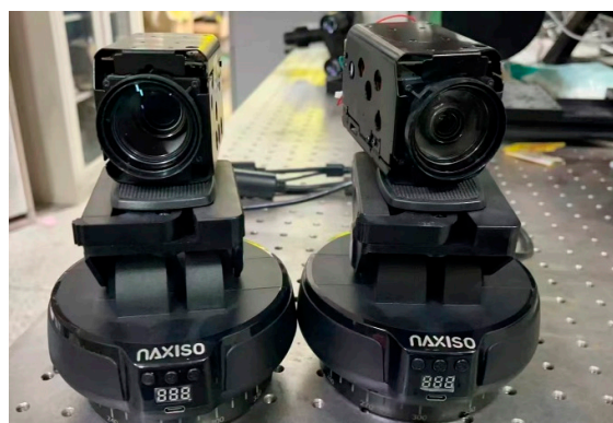
Figure 2. Experimental setup of the dual-FOV visible-infrared imaging system.
