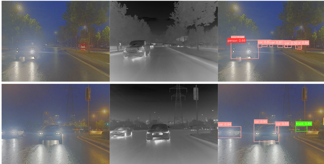
Figure 8. Representative failure cases of AQFS-Net under extreme conditions. ( Top row ): False positive caused by a misleading heat source. ( Bottom row ): False negative caused by severe optical and thermal reflections.
