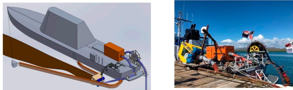
**Figure 6.** (Left) A design for a 5000 GPM pilot-scale version of the open-ocean, in-situ SOS pump-to-depth vessel that was designed, built, and tested. (Right) The constructed pilot vessel. A future fleet would comprise vessels with up to 50,000 GPM pumping capacity (multiple pumping systems in parallel).
