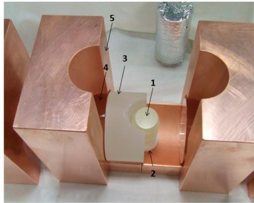
**Figure 7.**  $^{106}\text{CdWO}_4$  crystal scintillator (1), teflon stand for the  $^{106}\text{CdWO}_4$  crystal (2),  $\text{CdWO}_4$  crystal scintillators (3), quartz light-guide (4), and “internal” copper shield (5).
