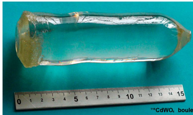
**Figure 9.** A large-mass crystal boule (~1.9 kg) of the enriched  $^{116}\text{CdWO}_4$  crystal was used in the experiment Aurora [91].
