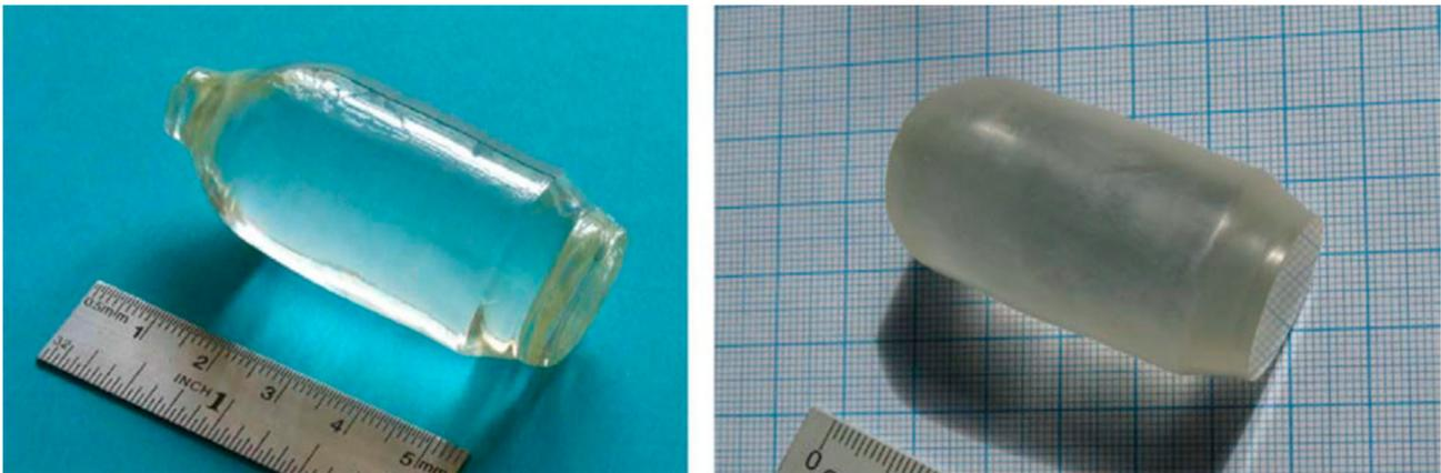
**Figure 4.** The crystal boule of  $^{106}\text{CdWO}_4$  (231 g) was grown by the low-thermal-gradient Czochralski technique (left).  $^{106}\text{CdWO}_4$  crystal scintillator (216 g) with diffused surface for better light collection (right). The figure was taken from [71].
