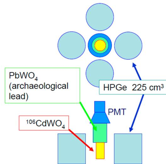
**Figure 5.** A scheme of the experimental GeMulti set-up with  $^{106}\text{CdWO}_4$ .
