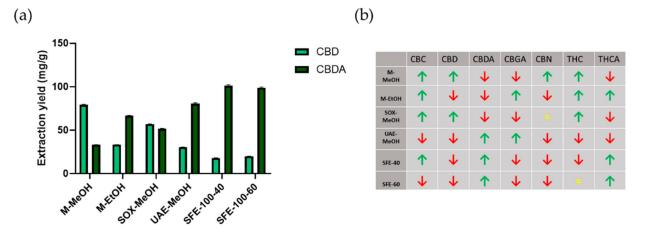
**Figure 2.** Comparison of cannabinoid extraction yields with different extraction methods. Panel (**a**) shows the amounts of CBD and CBDA obtained with different extraction methods (data are means  $\pm$  SD from n = 3 replicate measurements), and panel (**b**) shows the trends of all cannabinoids analysed across extraction methods tested compared to the average (= means as the average,  $\uparrow$  above average, and  $\downarrow$  below average).
