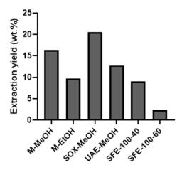
**Figure 1.** Extraction yield (EY) with different extraction methods (maceration with methanol— M-MeOH, maceration with ethanol—M-EtOH, Soxhlet extraction with methanol—SOX-MeOH, ultrasound-assisted extraction—UAE, supercritical CO<sub>2</sub> extraction at 100 bar and 40 °C—SFE-100-40, supercritical CO<sub>2</sub> extraction at 100 bar and 60 °C—SFE-100-60). Data are expressed as weight percentage (wt %) of the extracts obtained per 100 g of dry flower material.
