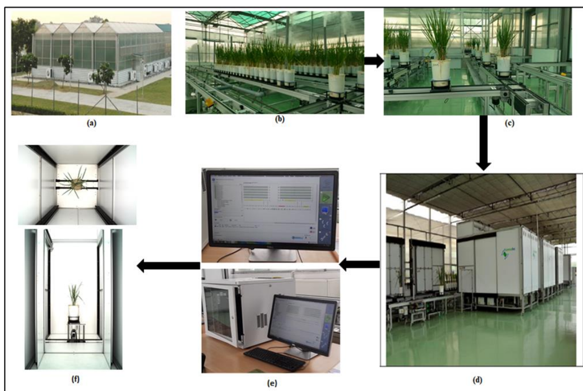
Figure 1. A plant-to-sensor type, high throughput plant phenotyping facility at Nanaji Deshmukh Plant Phenomics Centre (NDPPC), Indian Council of Agricultural Research–Indian Agricultural Research Institute, and their different components for the experimental setup, representing a general workflow: (a) NDPPC, external view; (b) rice plants in pots, transplanted inside the climate-controlled greenhouse; (c) rice plants are transported on carriages to the imaging chamber; (d) automatic imaging chambers, each chamber is equipped with a different sensor of interest, in this case, RGB; (e) monitoring and work station equipped with software; (f) image of a rice plant, top view and side view of the rice plant after imaging.
