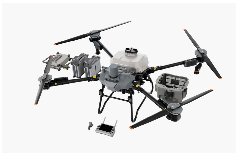
Figure 3. DJI T60 plant protection UAV. Note: The nozzle is located beneath the ends of the two rear rotors. The spray nozzle is located in the region affected by the downwash of the rotor, so after the droplets leave the centrifugal atomization device, they are affected by the rotor-induced airflow.
