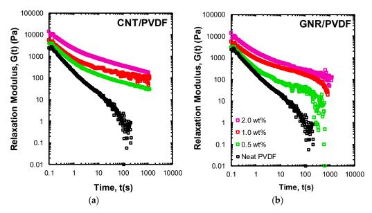
**Figure 3.** Stress dissipation upon application of a finite strain of  $\gamma = 10\%$  for (a) CNT/PVDF and (b) GNR/PVDF nanocomposite samples at different concentrations at 240 °C. The stepper motor response time is 0.1 s.
