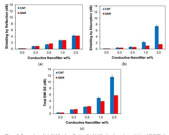
**Figure 5.** Comparison of **(a)** shielding by reflection, **(b)** shielding by absorption and **(c)** total EMI SE of CNT/PVDF and GNR/PVDF nanocomposites.
