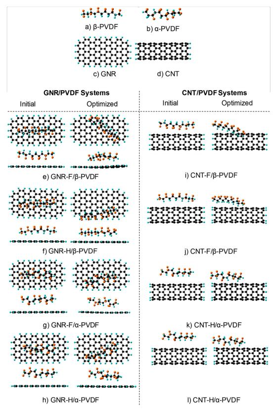
Figure 1. Optimized geometries of (a)  $\beta$ - polyvinylidene fluoride (PVDF), (b)  $\alpha$ -PVDF, (c) graphene nanoribbon (GNR), and (d) carbon nanotube (CNT). Initial and optimized structures of (e-h) GNR/PVDF (left side) and (i-l) CNT/PVDF (right side). The atoms in black, blue and orange correspond to carbon, hydrogen, and fluorine, respectively.
