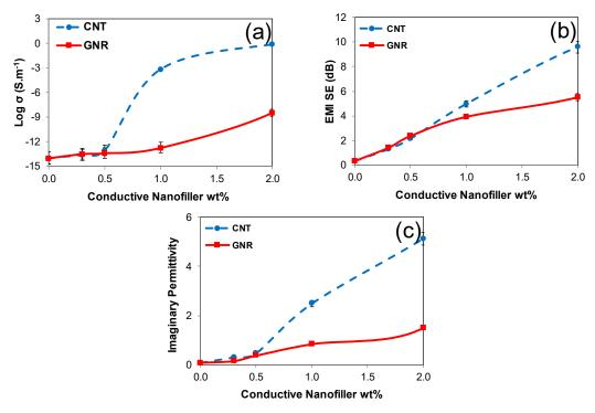
**Figure 4.** (a) Electrical conductivity, (b) electromagnetic interference (EMI SE) and (c) imaginary permittivity over the X-band (8.2–12.4 GHz) of parent CNT and GNR nanocomposites.
