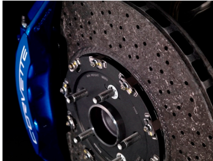
Figure 16. The braking system of corvette made of carbon–ceramic, which saved 4.9895 kg replacing iron, reproduced from [210] under open access license.
