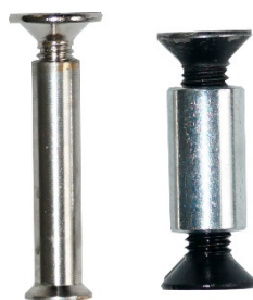
Figure 3. Used screws: (left) sleeve bolt (sb) and (right) a sleeve with screws from both sides (sl).
