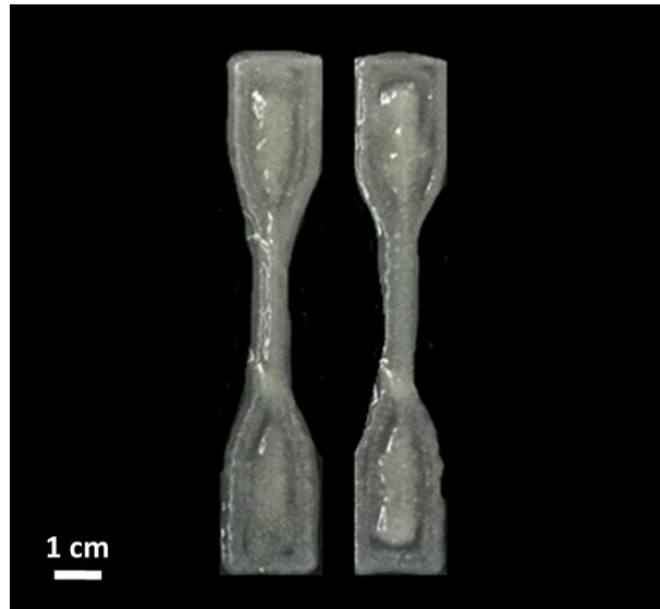
Figure S2. Liquid deposition modelling of 7 wt % CNF suspension followed by a standard tensile specimen 3D model according to the ASTM D638 Type IV (printing and slicing profiles; nozzle diameter: 1.21 mm; printing speed: 30 mm/s; extrusion speed: 3 mm/s; build plate temperature: 50 °C).
