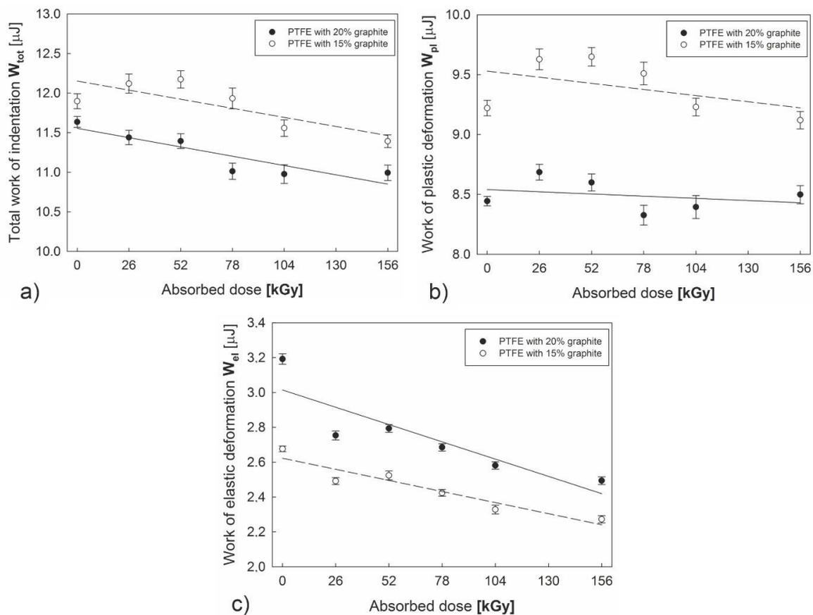
**Figure 7.** Changes in the work of indentation of PTFE with different graphite additions subjected to an absorbed dose of electron beam irradiation: the total work of indentation— $W_{tot}$  (a), the work of plastic deformation— $W_{pl}$  (b), and the work of elastic recovery  $W_{el}$  (c).
