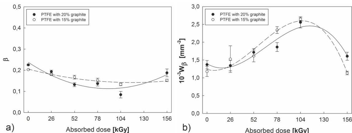
**Figure 9.** The effect of an absorbed dose of electron beam irradiation dose on the coefficient of the micromechanism of PTFE abrasive wear— $\beta$  (a) and the abrasive wear coefficient— $W_{\beta}$  (b).
