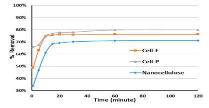
**Figure 6.** Contact time effect on tetraconazole removal by nanocellulose, Cell-F, and Cell-P (initial concentration ( $C_0$ ) = 10 ppm, adsorbent dose = 10 mg, solution volume = 10 mL, pH = 7, and temperature = 20 °C).
