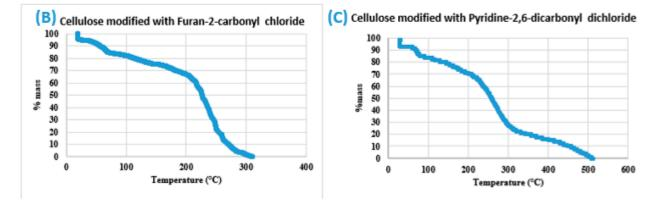
**Figure 5.** TGA analysis results for (**A**) Cellulose nanocrystal, (**B**) Cellulose modified with Furan-2-carbonyl chloride (Cell-F), (**C**) Cellulose modified with Pyridine-2,6-dicarbonyl dichloride (Cell-P).
