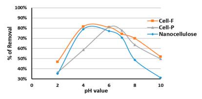
**Figure 7.** pH effect on tetraconazole removal by nanocellulose, Cell-F, and Cell-P ( $C_{\rm I} = 10$  ppm, time = 20 min, adsorbent dose = 10 mg, solution volume = 10 mL, and temperature = 20 °C).
