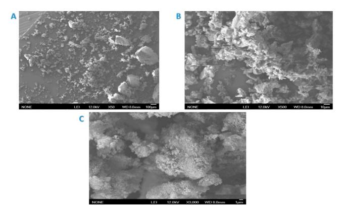
Figure 3. SEM images of Cell-F at three different magnifications: (A) 100 µm, (B) 10 µm, and (C) 1 µm.
