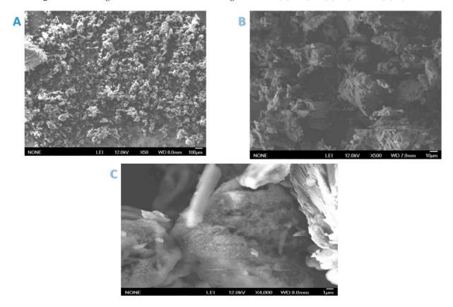
**Figure 4.** SEM images of pyridine-2,6-dicarbonyl dichloride (Cell-P) at three different magnifications: (**A**) 100  $\mu$ m, (**B**) 10  $\mu$ m, and (**C**) 1  $\mu$ m.
