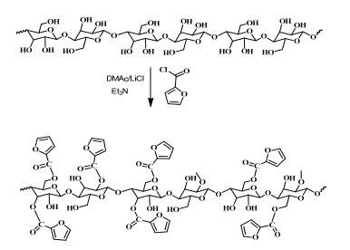
Scheme 1. Cellulose acylation with furan-2-carbonyl chloride.
