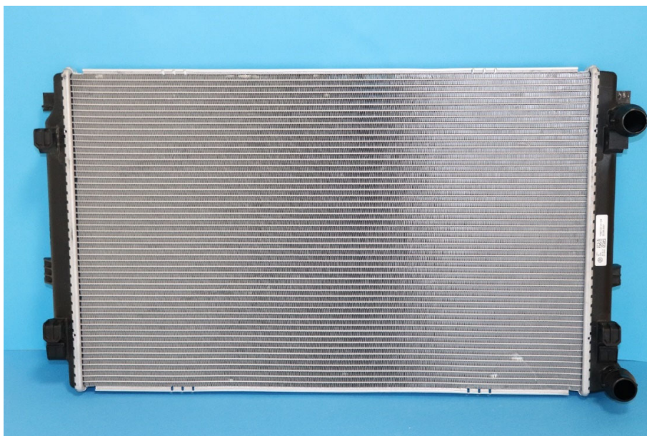
Figure 5. Aluminum radiator from Skoda Octavia used for comparison tests.
