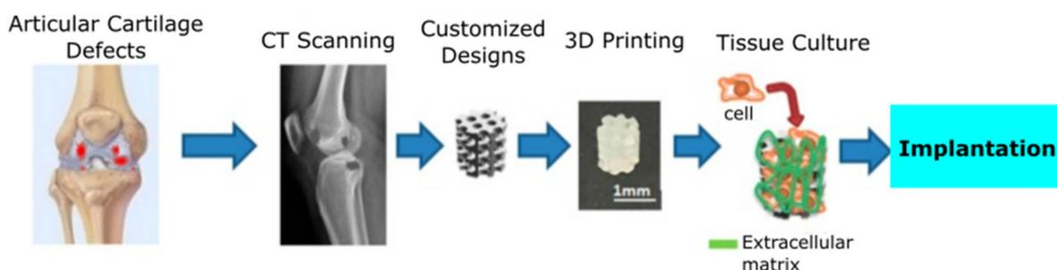
**Figure 14.** Schematic representation shows the 3D Printing of Water-Based Light-Cured Polyurethane with Hyaluronic Acid scaffolds for Cartilage Tissue Engineering Applications (Reproduced with permission from [114] CC-BY license, 2017).
