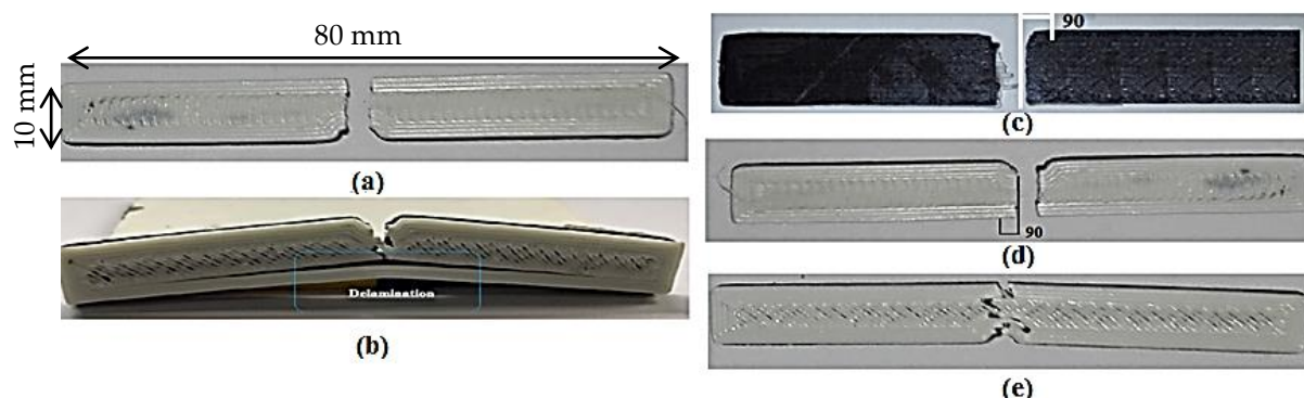
Figure 7. Fractures in C-PLA/ABS hybrid composite: (a) Both laminates fractured without any delamination; (b) Delamination of boundary wall; (c) Brittle fracture in C-PLA lamina with RA of 0^\circ/90^\circ and 45^\circ/-45^\circ ; (d) Brittle fracture in ABS lamina with RA of 0^\circ/90^\circ ; (e) Ductile fracture in ABS lamina with RA of 45^\circ/-45^\circ .
