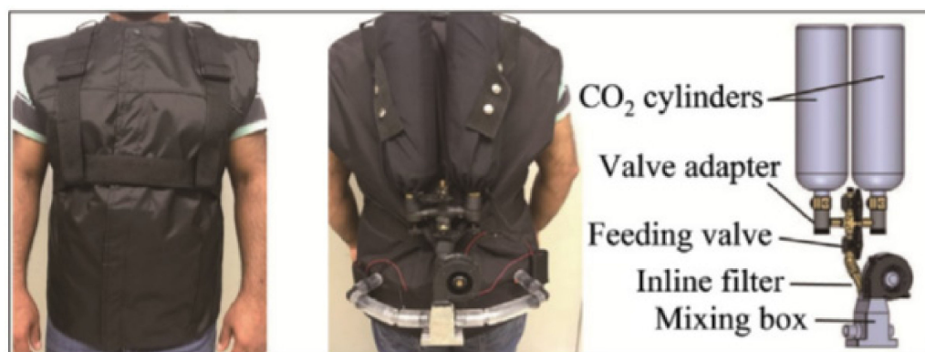
Figure 5. The air treatment system of the cooling garment with front view and back view. The prototype is composed of three parts: the layers forming the garment, the air treatment system, and the distribution channels. Reproduced with permission [249]. Copyright 2019, Springer Nature.
