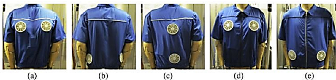
Figure 6. Small fans and openings on ventilated jacket located at different torso sites. The both fans are placed at (a) the upper back; (b) the lower back; (c) the mid back; (d) the chest (upper front); (e) the belly (lower front). Reproduced with permission [250]. copyright 2013 Elsevier.
