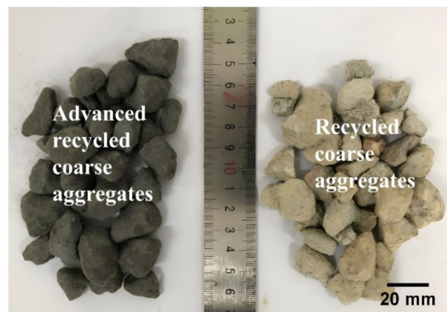
Figure 2. Coating appearance of RCA.
