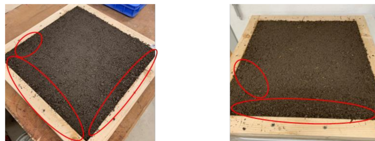
Figure 14. Cement bonded bark test specimens (430 × 430 × 20 mm) in a forming frame, nests with large bark particles marked in red.
