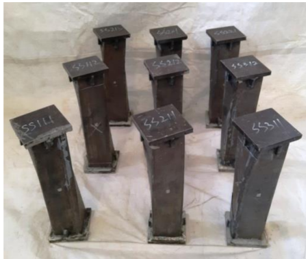
Figure 6. Square section specimen after flexural-torsional test.
