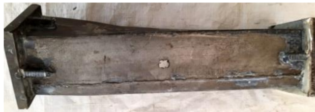
Figure 4. Failure model of steel tube.
