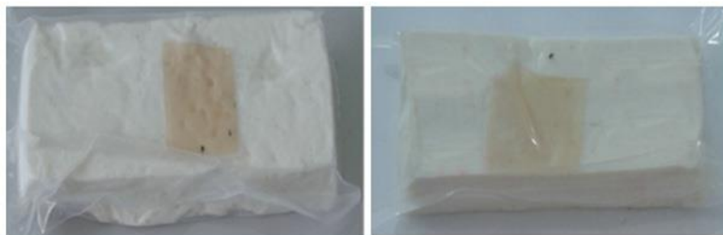
Figure 2. Color change in a pH-sensitive composite film produced from anthocyanins-loaded PVA–chitosan–gelatin for monitoring the spoilage of ricotta cheese during refrigerated storage: (left) 1 day (right) 7 days [73].
