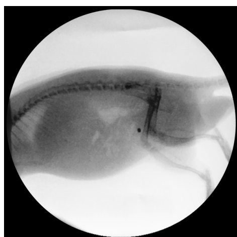
Figure 11. X-ray image of a rat, intravesical implant (2 × 2) mm, Elastollan + barium sulphate + a-C:H/Cu-multilayer coating. The selected concentration of 25% barium sulphate in the base material shows sufficient X-ray contrast. X-ray C-arm, Ziehm Vista, Zoom 2, 11 cm, Ziehm Imaging GmbH, Berlin, Germany.
