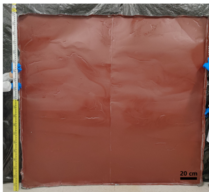
Figure 8. Image of the actual 2 m × 2.2 m flame-retardant coating.
