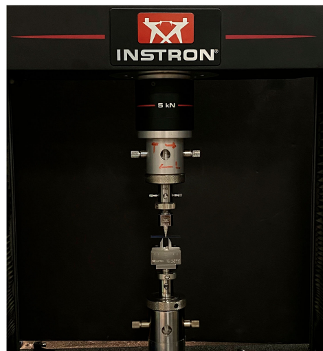
Figure 4. Three-point testing using Instron 5965 system (Instron, Canton, MA, USA).
