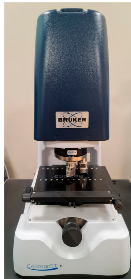
Figure 6. Surface roughness evaluation using Bruker Contour GTK (Bruker nano GmbH, Berlin, Germany).
