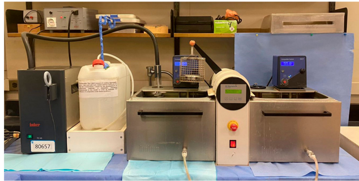
Figure 3. Thermocycler 1100 (SD-Mechatronik, Westerham, Germany).
