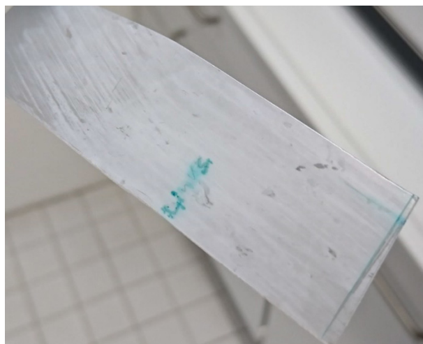
Figure 13. Hazing of CA sheet material at a humidity of below 20% RH.
