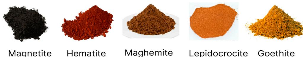
**Figure 5.** Visual appearance of iron oxides.
