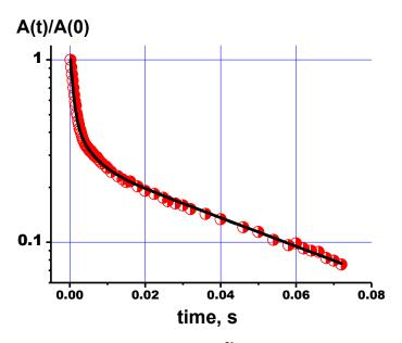
**Figure 11.** Relaxation decay of the <sup>31</sup>P NMR signal for the PVP-HA. White/red circles are the experimental data. Black line is the approximation according to Equation (2) with the parameters listed in Table 5.
