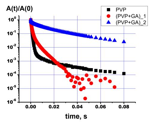
**Figure 9.** Relaxation decay curves of protons of NMR signals for PVP (black squares) and PVP-HA (red circles for protons with chemical shift 4.7 ppm and blue triangles for the signal at -2.15 ppm).
