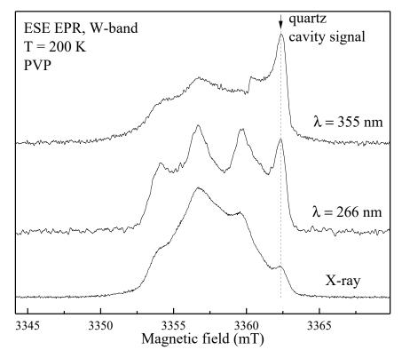
**Figure 6.** Photo-induced (using lasers with the wavelengths of 355 and 266 nm) and X-ray induced ESE EPR spectra at T = 200 K of PVP in the W-band. The dotted vertical line shows the signal from the quartz tube of the sample holder.
