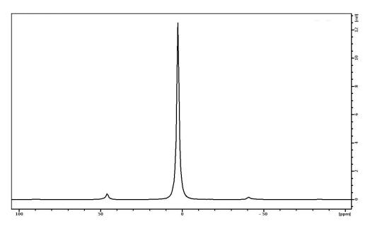
**Figure 10.**  $^{31}$ P NMR spectrum of PVP-HA. The sample rotation frequency is 7 kHz.
