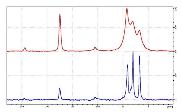
**Figure 8.** MAS-NMR spectra of  ${}^{13}C\{{}^{1}H\}$  cp (red) and hpdec (blue) of the PVP. The rotation frequency of the sample is 7 kHz.
