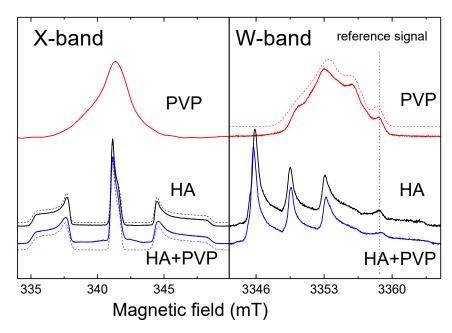
**Figure 5.** EPR spectra obtained by detecting the ESE of samples after X-ray irradiation: X-band in the the left panel, W-band in the right panel. The red lines show the spectra of PVP, the black lines the spectra of HA, and the blue lines the spectra of PVP-HA. The dotted lines show the approximations of the EPR spectra. The approximation parameters are given in Table 1.
