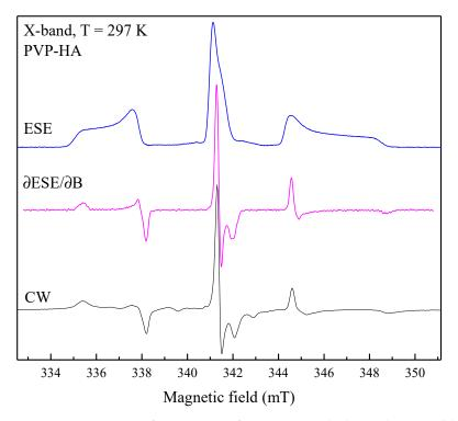
**Figure 4.** Comparison of EPR spectra of PVP-HA sample detected via ESE (blue upper curve) and cw (black lower curve) after X-ray irradiation in the X-band at T = 297 K. Middle curve was obtained by differentiating the ESE EPR spectra.
