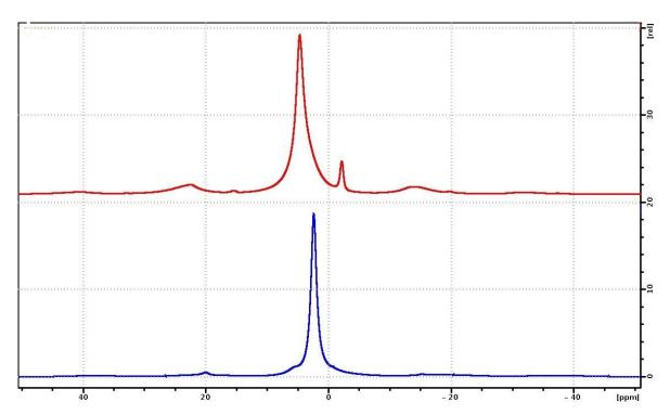
Figure 7. <sup>1</sup>H NMR spectra of PVP (blue curve) and PVP-HA (red curve) samples.
