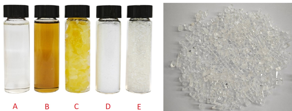
Figure 25. Intermediate products of poly(lactide) synthesis: A—lactic acid; B—lactic acid oligomers; C—raw lactide; D—purified lactide; E—poly(lactide) pellets obtained using a laboratory extruder.
