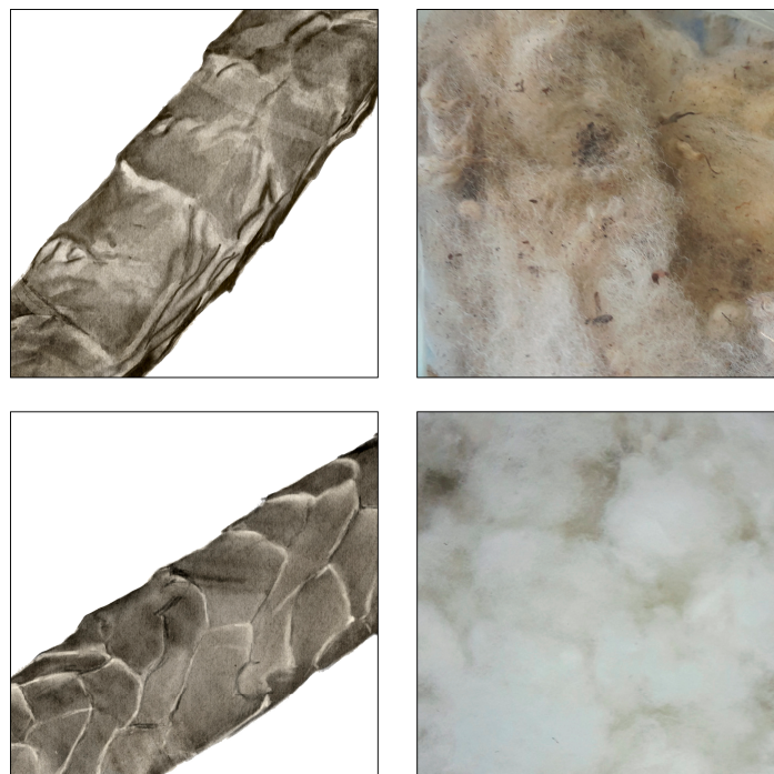
Figure 3. The surface appearance of sheep wool before (up) and after (down) scouring in an ultrasonic bath (Adapted by Z. Braniša from [9]).
