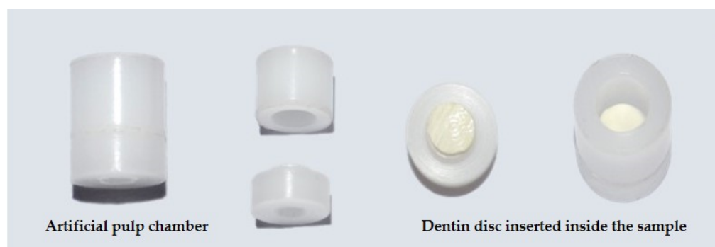
Figure 2. Artificial pulp chamber device.
