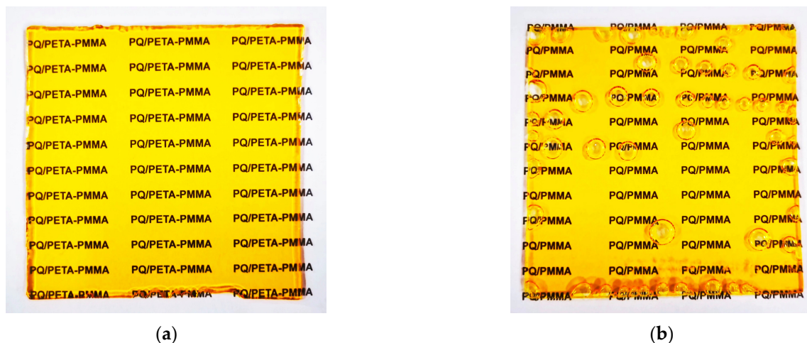
Figure 2. (a) PQ/PETA-PMMA molding case (2 h baking). (b) PQ/PMMA molding case (20 h baking).
