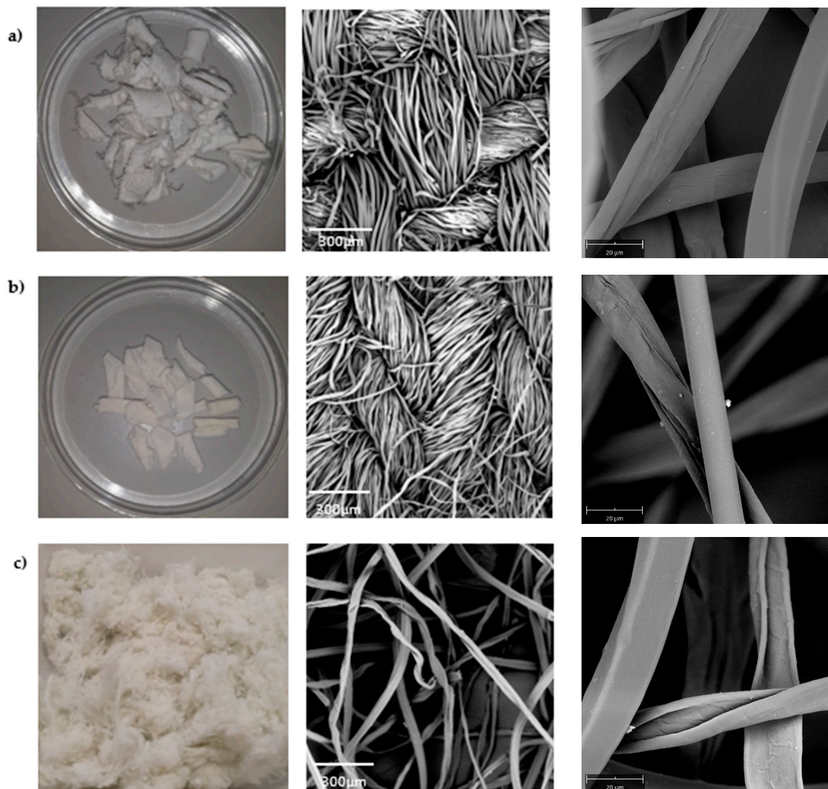
Figure 2. Photographs (left) and SEM micrographs ((centre) and (right)) of samples of (a) woven fabric waste, (b) knitted fabric waste, and (c) mixed waste.
