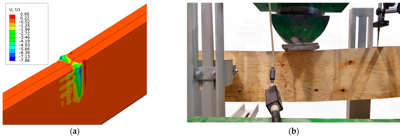
Figure 14. (a) Typical deformation of LVL at the concentrated load; (b) corresponding failure mode.
