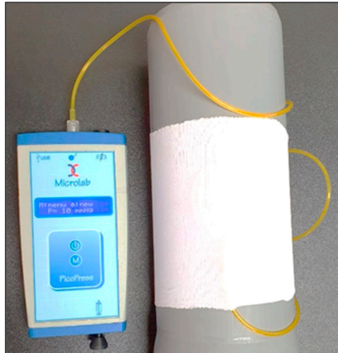
Figure 4. Positioning of the material over a cylinder and connection to the PicoPress apparatus.
