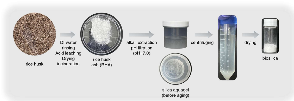
Figure 1. Schematic of extraction biosilica process from rice husk ash by alkali extraction and titration.
