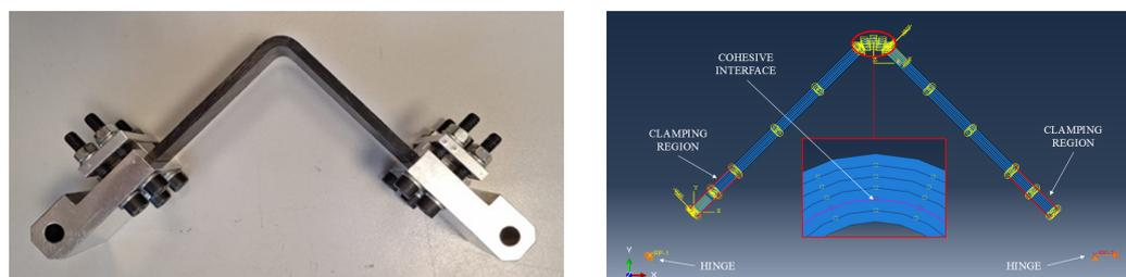
(a) Curved beam specimen with hinges.
